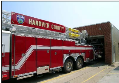
Assigned ladder truck does not fit
